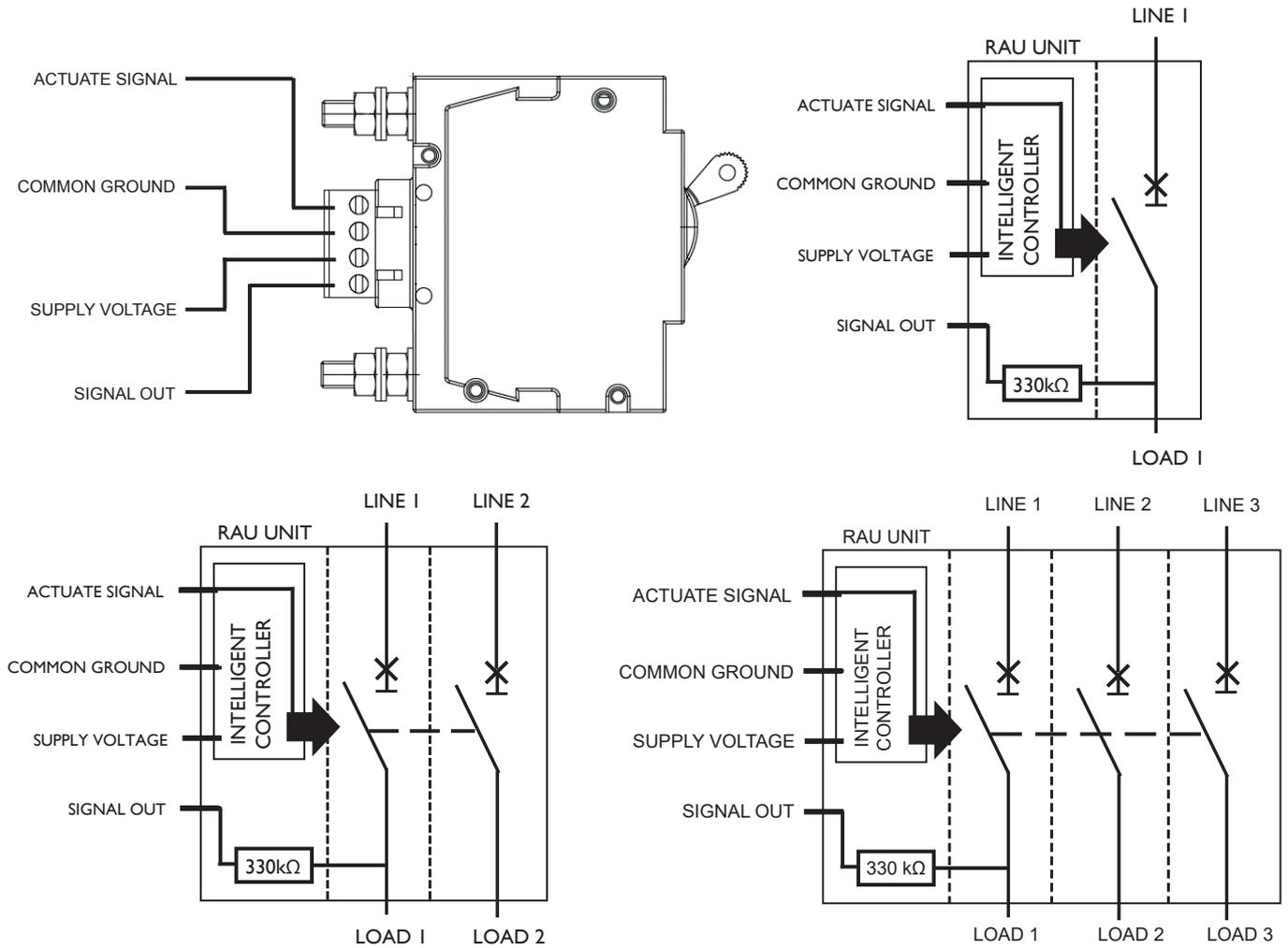
Note: Signal out only provides status indication of the adjacent pole through a 330 kΩ resistor.
